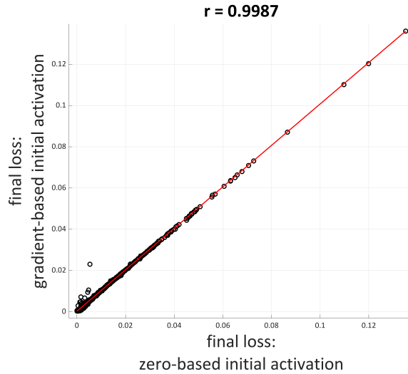
Fig. 13. Scatterplot of by-trial losses of zero- and gradient-based-initialization strategies. Red line is the function x = y . The proximity of points to this line indicates a high degree of correlation.
